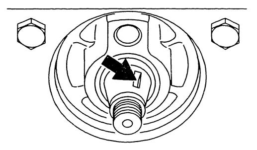
Slip drive coupling onto drive shaft. Attach plunger-stroke measuring device KDEP 1085 (see picture) and set dial indicator to "zero" in BDC position of distributor pump plunger.
